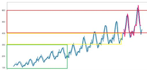
Figure 3. An illustration of a possible model predicting the probability of axle seal leaks in feedwater pumps. The blue line is the projected trend of a process variable, and the different colored boxes indicate an increased risk of a leak appearing.
