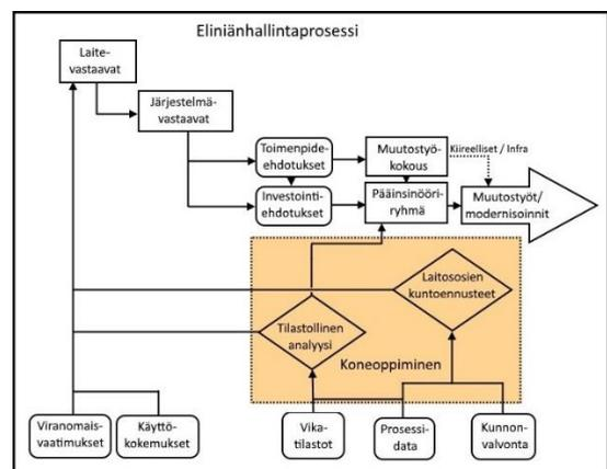
Figure 1: A simplified chart of the TVO lifecycle management process, where the orange background signifies the future place of machine learning. (Vaaheranta, 2018) [1]
