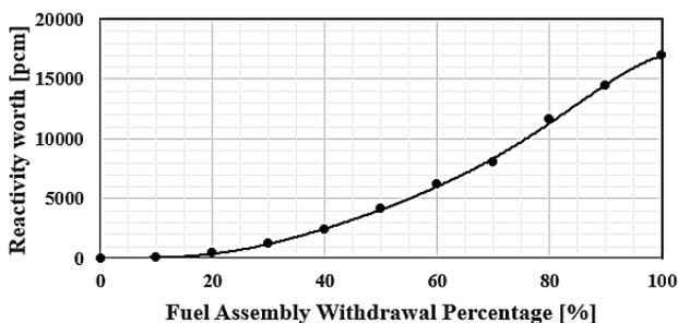
Figure 7: Fuel assembly reactivity worth of the 2-MW<sub>th</sub> LUTHER core.
