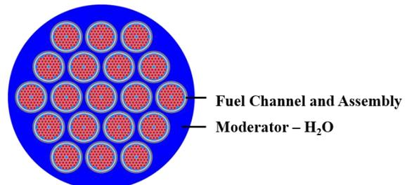
Figure 2: Schematic view of the 2-MW<sub>th</sub> LUTHER core.
