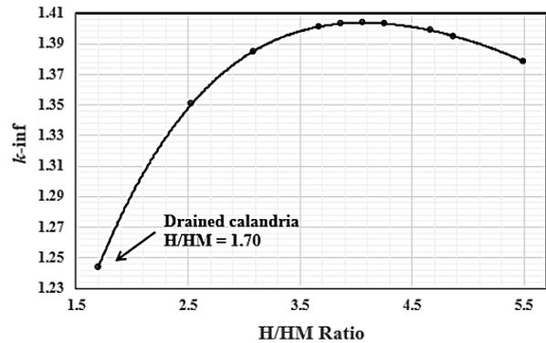
Figure 3:  $k_{\infty}$  of a fuel assembly as a function of H/HM ratio with a fuel rod pitch of 0.96 cm and an assembly pitch of 10.5 cm.
