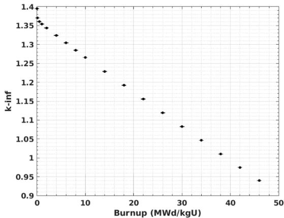
Figure 5:  $k_{\infty}$  of a fuel assembly without burnable absorbers as a function of burnup.
