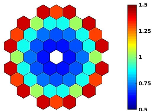
Figure 4: Normalized power distribution in a single fuel assembly with identical 4.95%-U enriched fuel rods.
