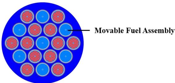
Figure 6: One possible configuration for the movable fuel assemblies.
