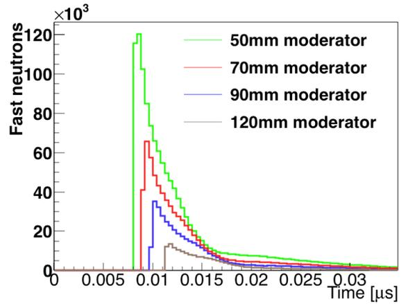
Figure 3. The MC simulation results show how the polyethylene moderator thickness affects the arrival-time distribution of fast ( $E_n = 1\text{--}2.5$  MeV) neutrons within an unknown-object volume.
