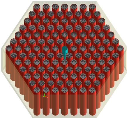
Figure 1. The simulated geometry of a VVER-440 reactor fuel assembly that is used in the GEANT4 simulations. The fuel pellets, in grey, are enclosed in the red fuel rods while the blue rod in the middle marks the position of a water channel.
