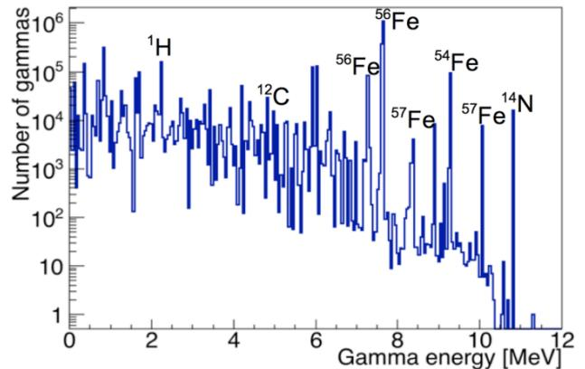
Figure 4. The emission spectrum of gamma rays resulting from neutrons impinging on a TNT-filled artillery shell as calculated in the MC simulation. The most prominent peaks in the energy spectrum are marked with their nuclide of origin.
